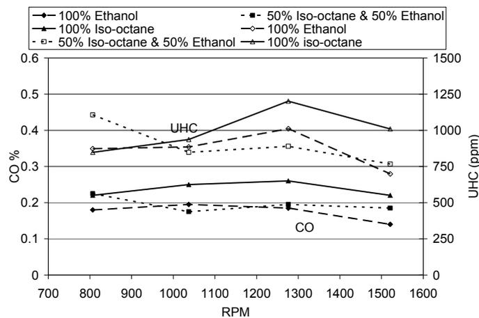
Fig. 14. Carbon monoxide and UHC emissions
