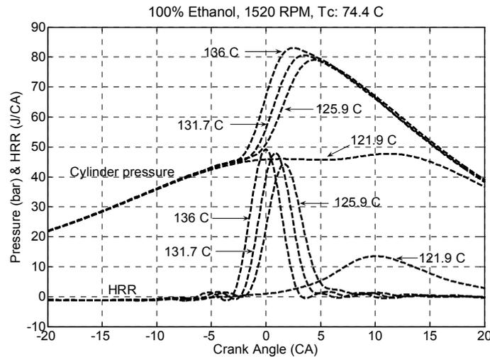
Fig. 8. Cylinder pressure and rate of heat release at different intake charge temperatures (1520 RPM, 100% Ethanol)
