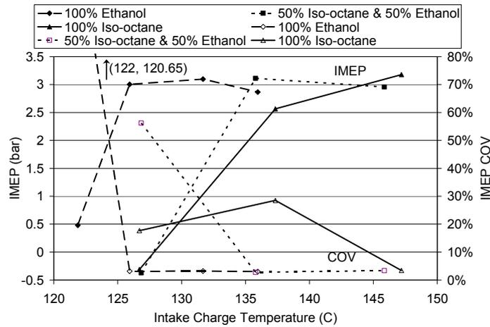
Fig.10. IMEP and  $COV_{IMEP}$  at 1275 RPM
