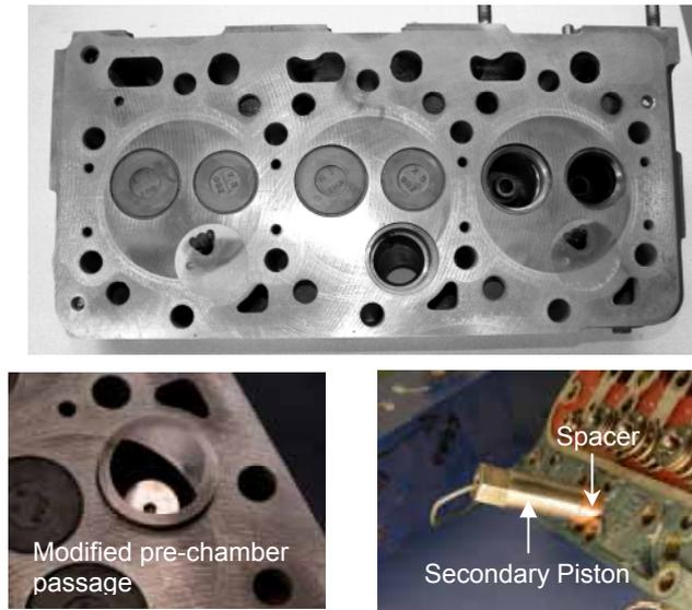
*Fig. 2. Engine head with secondary piston and spacer arrangement, [11].
