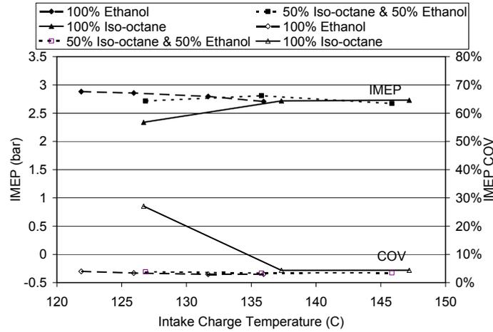
Fig. 9. IMEP and  $COV_{IMEP}$  at 1035 RPM
