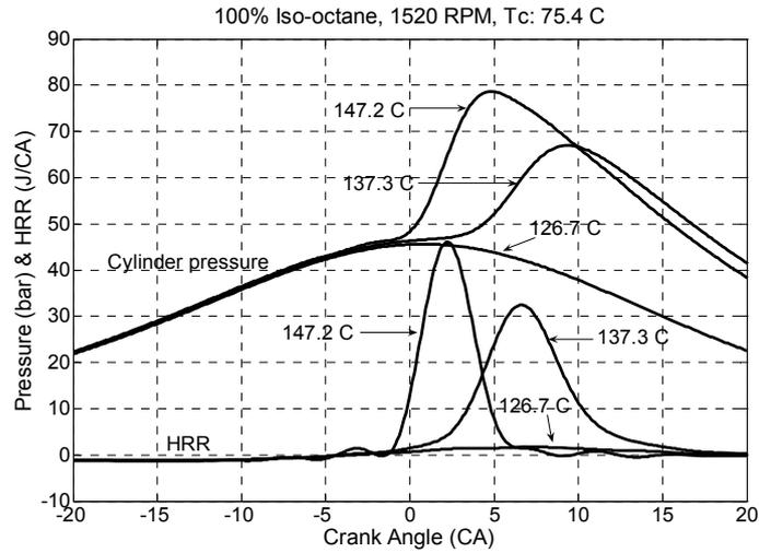
Fig. 6. Cylinder pressure and rate of heat release at different intake charge temperatures (1520 RPM, 100% Iso-octane)
