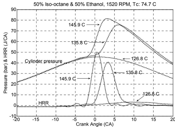
Fig. 7. Cylinder pressure and rate of heat release at different intake charge temperatures (1520 RPM, 50% Iso-octane and 50% Ethanol)
