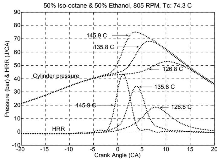
Fig. 4. Cylinder pressure and rate of heat release at different intake charge temperatures (805 RPM, 50% Iso-octane & 50% Ethanol)
