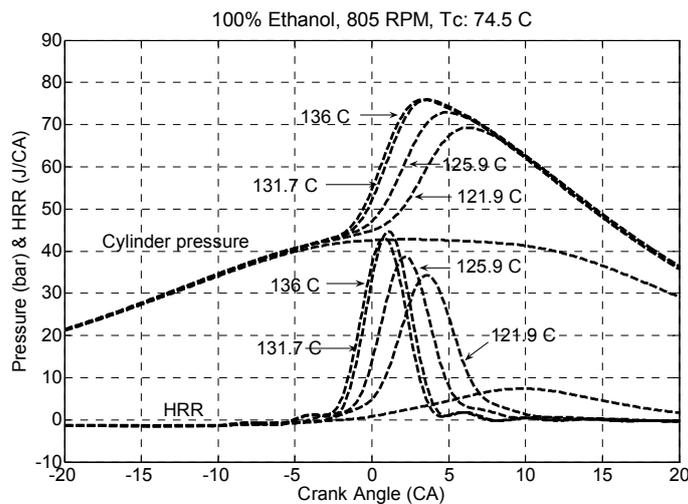
Fig. 5. Cylinder pressure and rate of heat release at different intake charge temperatures (805 RPM, 100% Ethanol)
