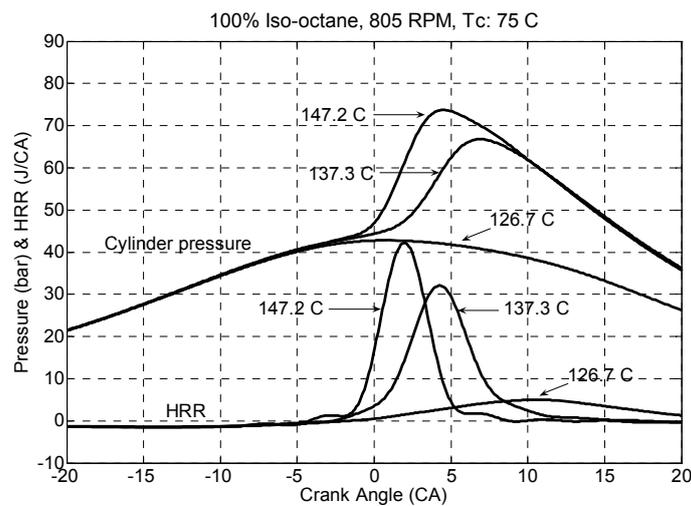
Fig. 3. Cylinder pressure and rate of heat release at different intake charge temperatures (805 RPM, 100% Iso-octane)
