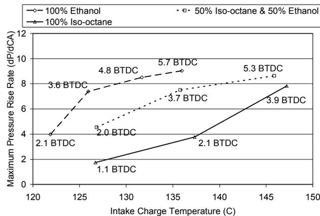
Fig.13. Maximum pressure rise rate with corresponding combustion on-set CA values at 1035 RPM
